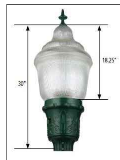
DECORATIVE POST-TOP LED LIGHTING FIXTURES MOUNTED 10FT ABOVE GRADE: SYSTEM SHOWN CONSISTS OF 7 LED FIXTURES, 61watt INPUT, 8.3k LUMEN OUTPUT, TYPE-3 LIGHT DISTRIBUTION, BUG RATING B2-U5-G5
