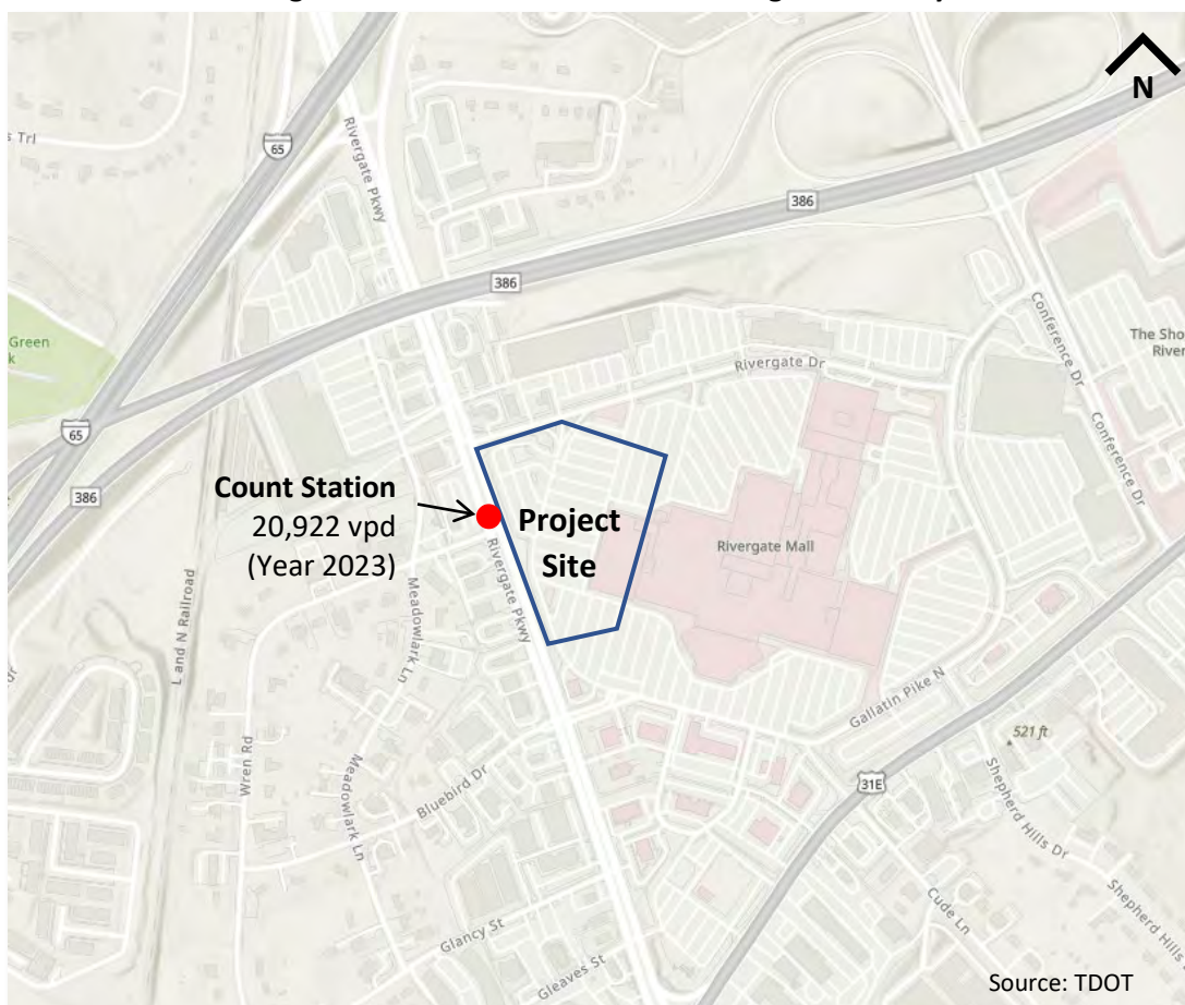
Figure 1: TDOT Count Station on Rivergate Parkway
