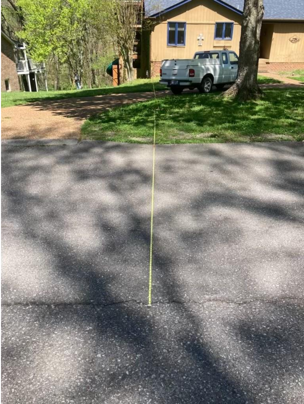
Close up of center of road to mark 25 ft to a point with a post placed under the tree to mark the 25 ft road frontage setback required.
