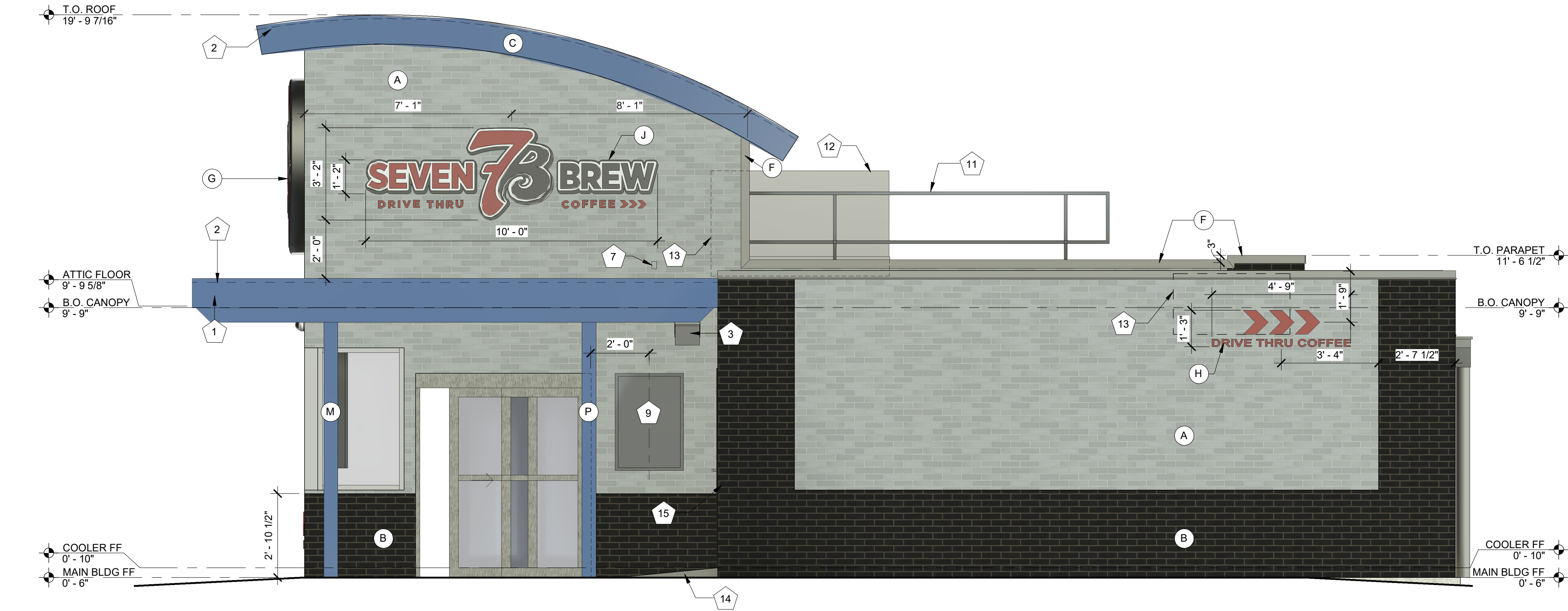
2 EXTERIOR ELEVATION - SOUTH W/ COOLER 3/8" = 1'-0"
